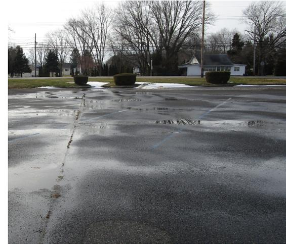
Parking spaces in the parking lot to the south of the building near the entrance can be converted to porous pavement to capture and infiltrate stormwater runoff from the parking lot. Two rain gardens can be installed at the back building's western entrance to capture and treat runoff from the roof. A preliminary soil assessment suggests that more soil testing would be required before determining the soil's suitability for green infrastructure.
